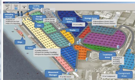
**Car Logistics:** The motivating case study is inspired by the operation of the sea port of Bremen, Germany. The port receives ships loaded with cars and has to organize their delivery. The operation of the system involves numerous entities (Ships, Cars, Gates, Landing Manager, Unloading Managers, Terminals, Treatment Areas, Delivery Managers, Delivery Gates, Trucks...), each responsible of specific tasks and characterized by its own needs and requirements.
